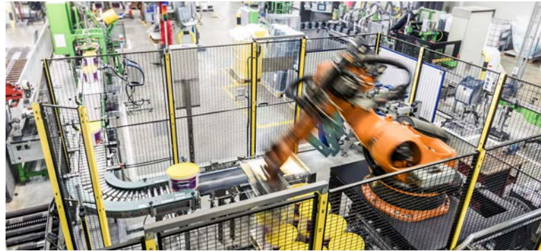
Fully automated robots take over the stacking of finished products on transport pallets.
