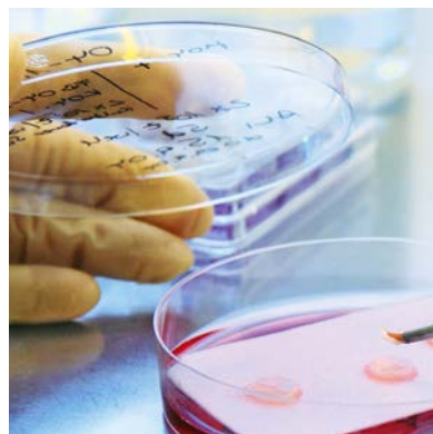
Substances can be applied to this full skin model developed by Henkel, in order to systematically assess their effect on skin tissue.
