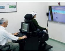
Our Research & Development teams have developed a special simulator that uses the latest virtual reality techniques to help train crane operators. Replicating the actual experience of working the crane through state-of-the-art graphics, sound systems, LCD projectors, and movement sensors help to improve the skills of inexperienced workers, and increases safety throughout our operations.
