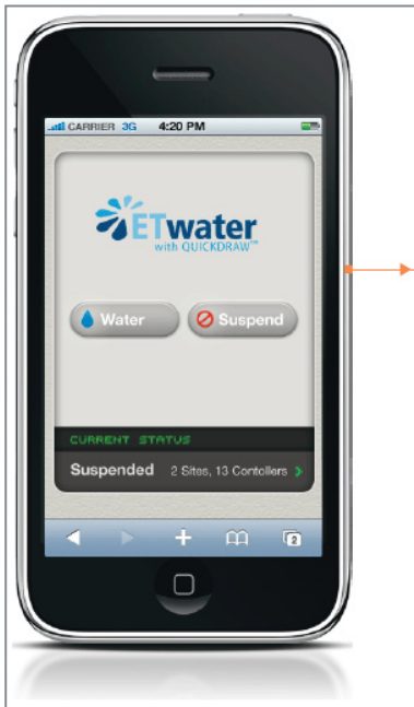
Figure 14: ET Water's QUICKDRAW mobile application allows users to operate irrigation systems remotely. (Source: ET Water)
