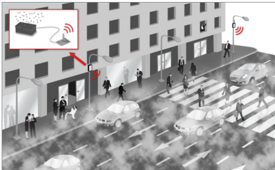
Figure 21: Libelium's Smart Cities platform includes wireless pollution monitoring sensors (Source: Libelium)
