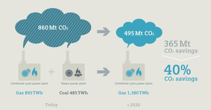
The coal-to-gas shift would lead to 365 Mt CO<sub>2</sub> savings from 2030 onwards
